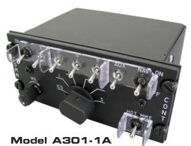
The A301-1A is an upgraded version of Andrea Systems C-6533 product which has been providing reliable service in a variety of helicopters, military and commercial aircraft for almost 40 years. This modernized version boasts a range of new features including digital switching, surface mount technology, and an option to add VOX.
